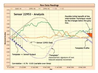
Sensor 22953 (grey line) is delivering the more consistent signal (the green plot suggested subsidence commencing in early March, which can't be root induced). Comparing the output with the characteristic signature of root induced clay shrinkage (above) we see (right hand side of plot) that there is initial cause for some cautious optimism, but we will see through June and July.
