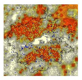
The only link that we could find was a geological one using our soils map 'in the alternative' provided a far better indication of the peril than any individual item of data. Above we have thematically mapped soils PI in the ranges 0-10, 10-20, 20-30, 30-40 and > 40. Yellow dots are clay shrinkage, blue dots are water claims.
