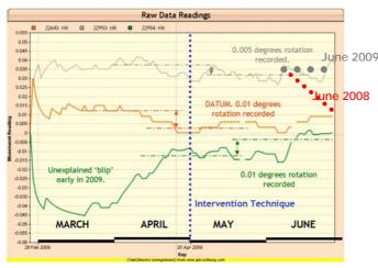
The treatment method will be reviewed taking into account our findings throughout 2009. The objective is to reduce the amplitude of movement, even though 2009 looks like being a drier year than 2008.
