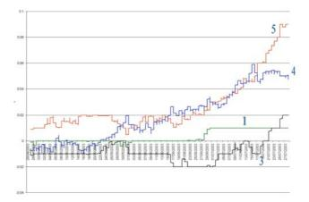
The amplitude of movement also varied. Sensors 4 & 5 rotated by about 0.09 degrees. Sensors 1 & 3, less at around 0.02 degrees but with a variable signature.
