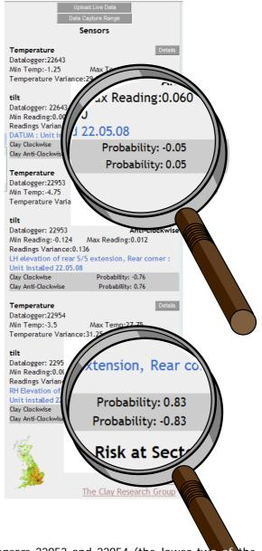
Sensors 22953 and 22954 (the lower two of the readings) show probabilities of 0.78 (max variance 0.124 degrees) and 0.83 (max variance 0.1 degrees) that the pattern of movement is due to root induced clay shrinkage. Anything above 0.7 has a very high confidence. In contrast, the datum has a probability of 0.05 with a max variance of 0.06 degrees.
